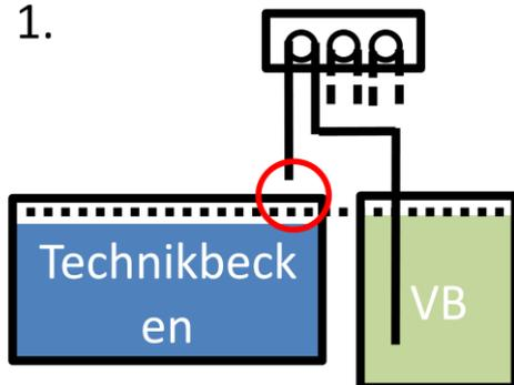
**Important:** The dosing pump and your outlets should always be above the top level of your Essential dosing solutions (1, 2 and 3). The outlet should also not be in contact with the aquarium water (red circle). The overall difference in heights should be minimal.
