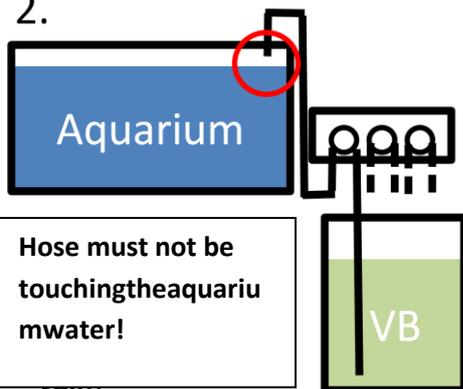
**Why:** If the pump is not positioned correctly the tubes may not be completely shut off when not dosing. If the dosing pump outlets are below the Essentials solutions levels in the storage containers, then siphoning can cause uncontrolled dosing
